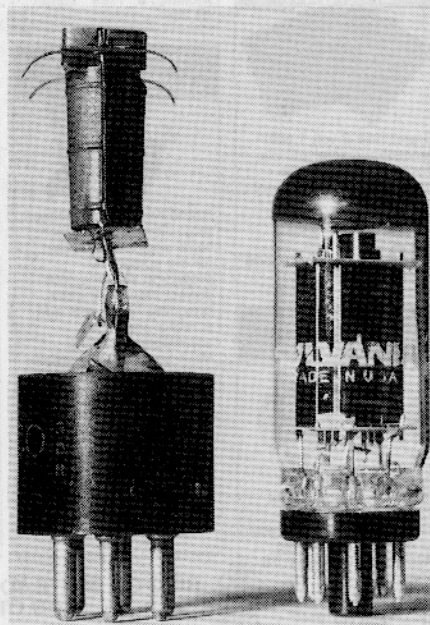
Fig.1: The internals of a traditional type 42 (left) show clearly how the 'press' with in-line element supports gave poor support. At right is a late-model Sylvania 6V6GTA, showing the 'button' type base which was first developed by RCA for the 'bullet' tube, and then used in the metal octal valves.
