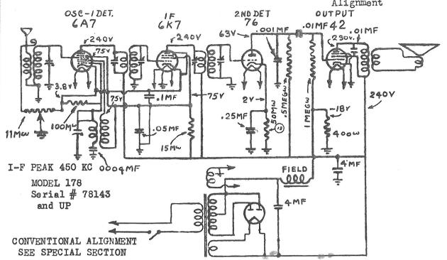
Align the I-F transformer trimmers at 450 KC.
