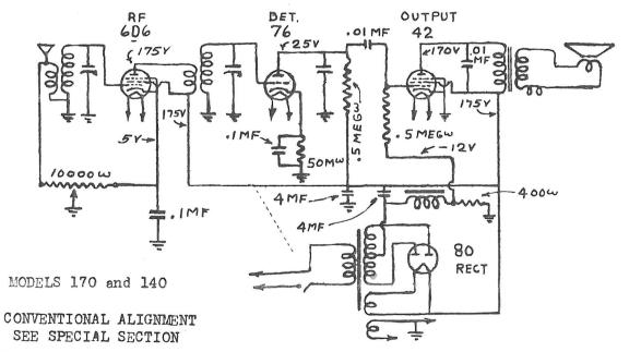
The generator is connected to the antenna of the receiver and set to 1400 KC. The trimmer of the front section of the variable condenser is then adjusted to maximum peak. The rear trimmer of the variable condenser (ANT) is next peaked to maximum.
