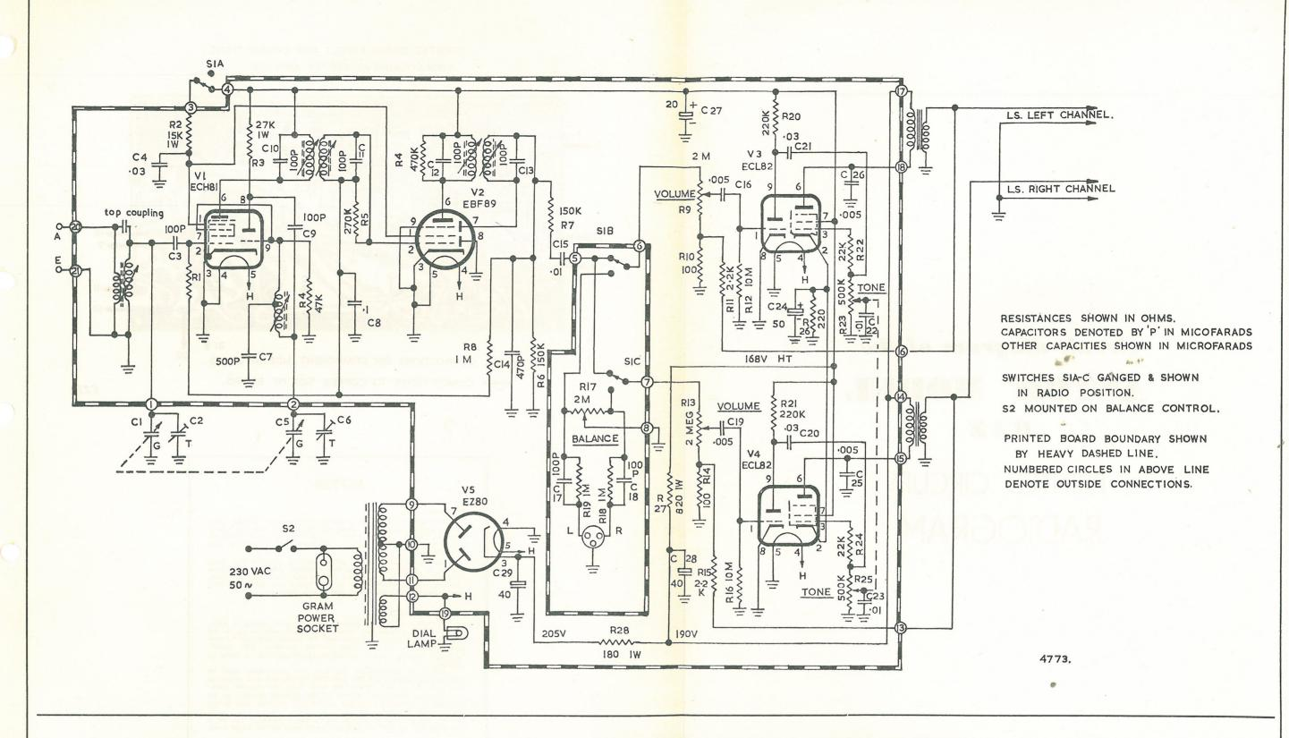
circuit diagram of Astor 'PRINTED CIRCUIT' Radiogram
