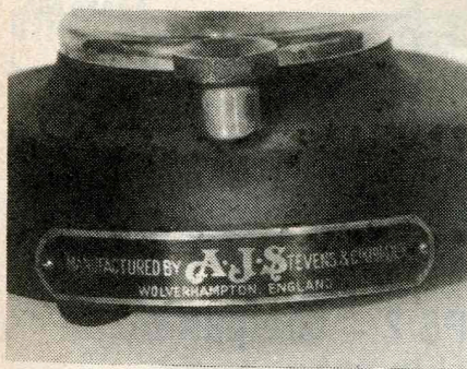
Not a piece of a vintage motor cycle, despite the name plate! The knurled knob is the diaphragm spacing control.
