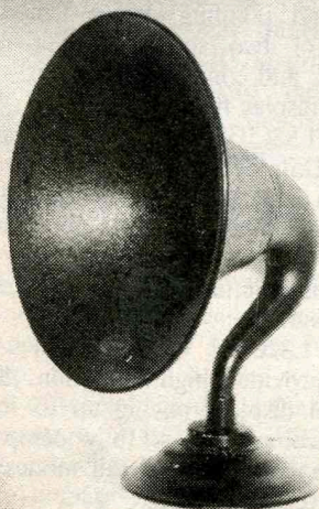
An American Atwater Kent model L. It has a spacing adjustment collar under the base.
