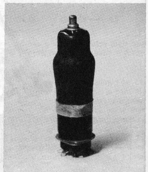
Fig.1C: After re-gluing the base and coating the wire with epoxy resin, cover the repair with a strip of tape or paper.
