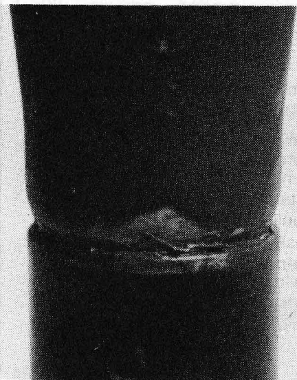
Fig.1A: A common problem with metallising. Not only has the base become loose, but the earthing wire has lost reliable contact with the shielding.
