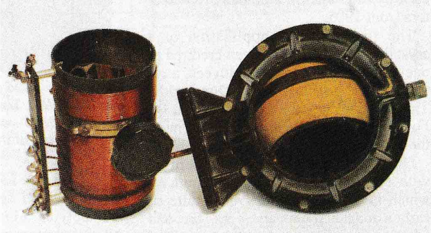
Fig.9: Variometers were frequently used as variable inductors for tuning in the better grade sets, such as the GEC model in Fig.3. They could also be used to provide variable coupling in double-tuned sets.
