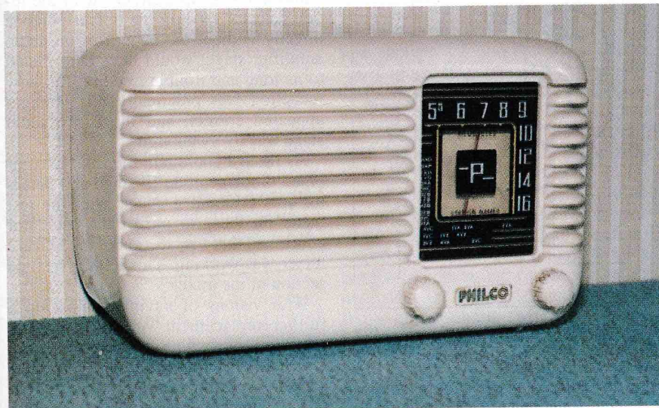
Fig.1: With only three Philips Noval valves plus rectifier, this little New Zealand made Philco receiver has a very basic circuit not unlike the 'Little General'. After 40 years of trouble-free service it developed a classic fault...
