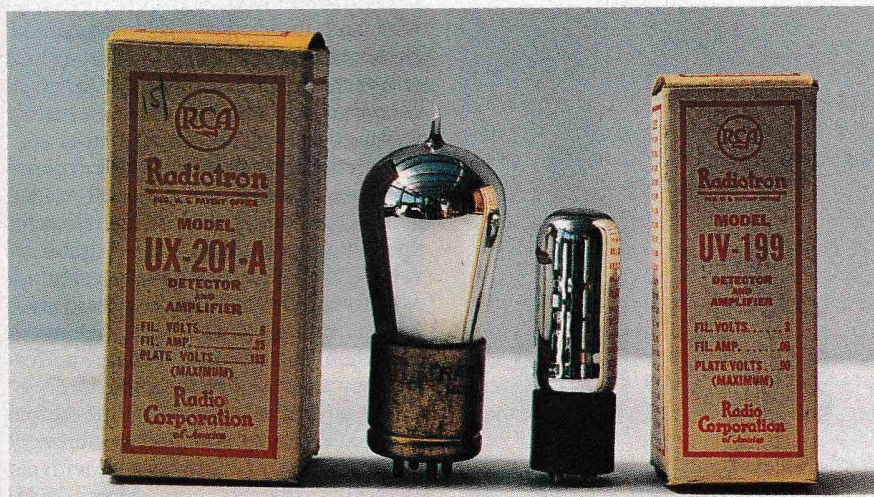
During the early and mid 1920's, the American scene was dominated by the '01A and '99. In contrast with the pure tungsten filament valves, these thoriated tungsten types needed heavy gettering.
