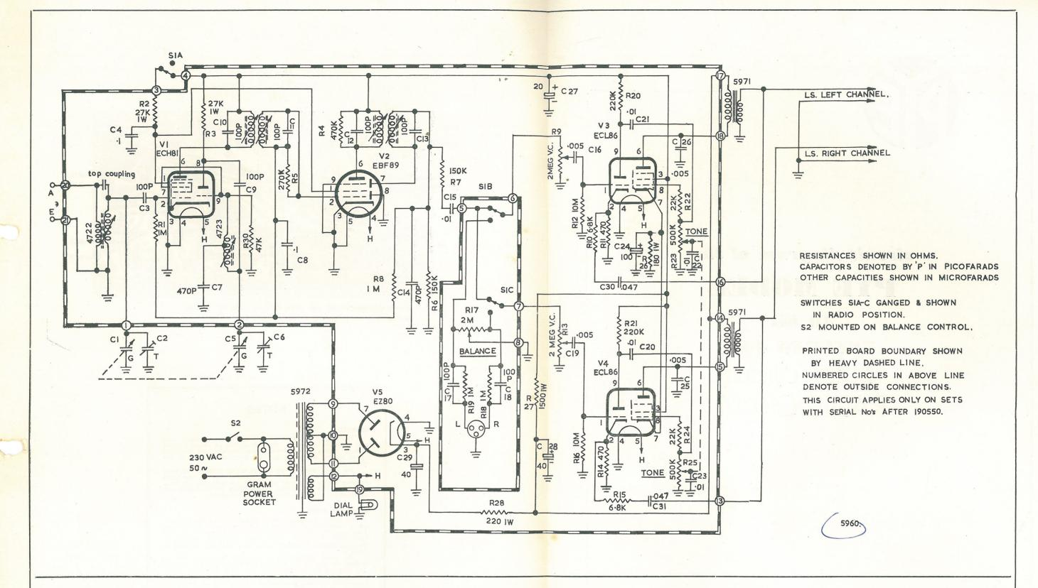
circuit diagram of Pye 'PRINTED CIRCUIT' Radiogram
