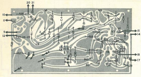
CONNECTIONS ON COMPONENT SIDE OF BOARD. CONNECTIONS TO COPPER SIDE OF BOARD.
