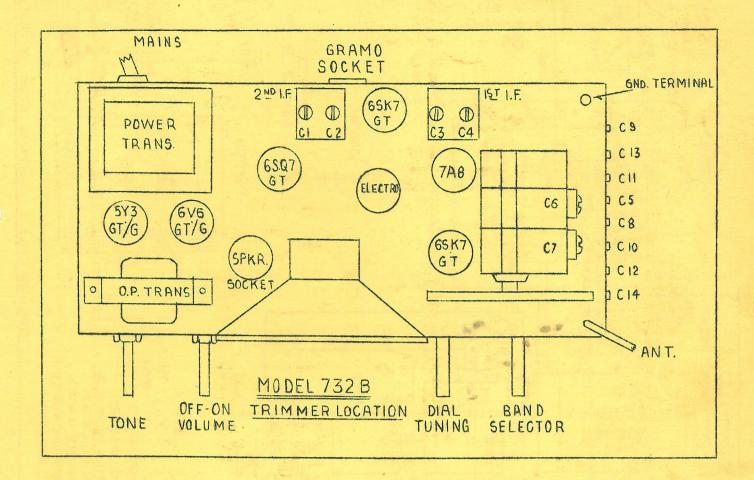
The model 732B is very similar to the previous models 732 and 732A but uses higher gain 6SK7 tubes. Other modifications include changes to the bandsproad series condensers, while the l.F. transformers have been altered to realise the extra amplification from the tubes.
