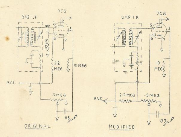
Remove 100 mmfd condenser from between diodes of 706
