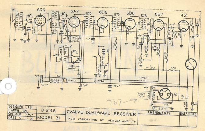
4. RESISTANCE TESTS: Where Measured. Power tran. primary Resistance in Ohms. Across power cord H.T. secondary Approx. 40 Each rectifier plate to ground Speaker, field "Fil" of speaker socket
