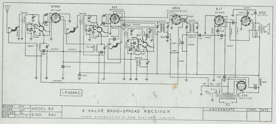
NOTE: Osram valves KTW61 and X65 can be replaced by their equivalents 6K7G and 6J8G respectively, without any alteration to the circuit.
