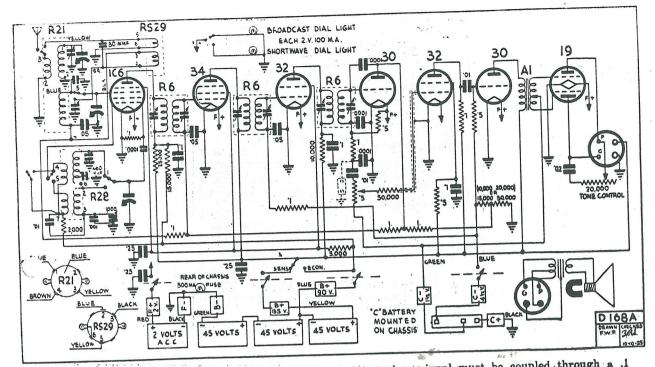
WARNING: When applying signal to grids of I.F. or mixer valves signal must be coupled through a .1 MF Cond. to avoid shorting Bias.
