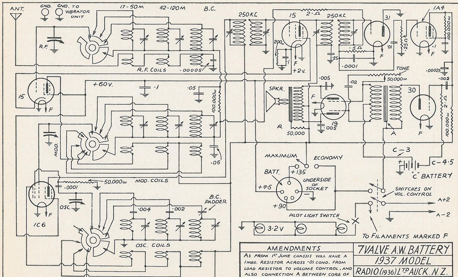
THE THREE SEGMENTS OF EACH SWITCH SECTION ARE SHOWN IN B.C. POSITION. ROTATE 30° TO LEFT FOR MEDIUM BAND, AND 60° TO LEFT FOR SHORT WAVE BAND.
