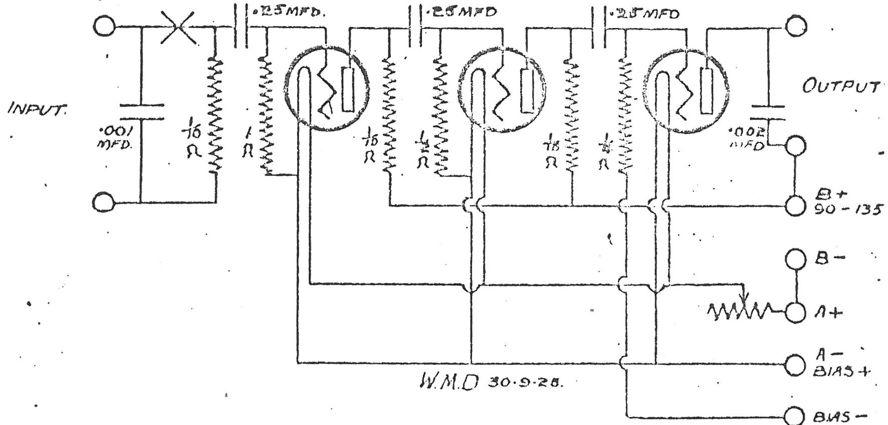
This three-valve amplifier adds no control to the set
