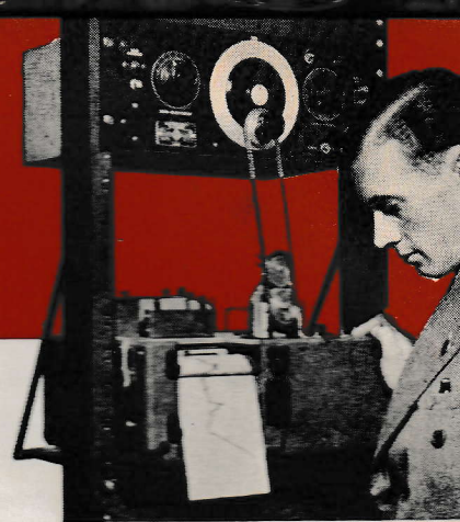
Taking a loudspeaker response curve
