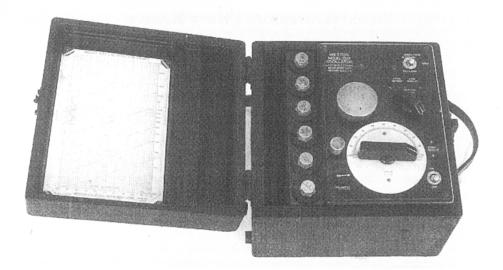
Above: Weston Modulated Oscillator model 692 in its carrying case. The output lead (not shown) is carried in the slot alongside the six coils which, in use, are plugged in under the removable metal cap above the dial. The attenuator control is to the right of this cap.
