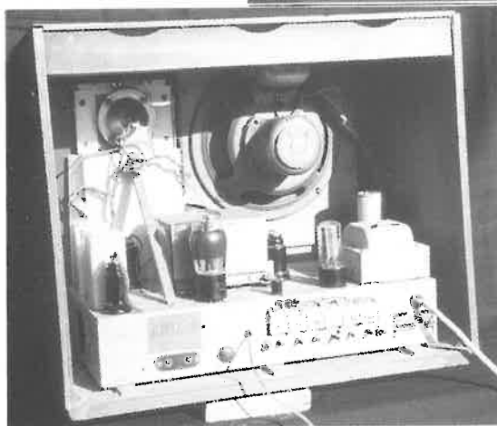
Rear View of Skyscraper EA showing trimmer capacitors for station selection
