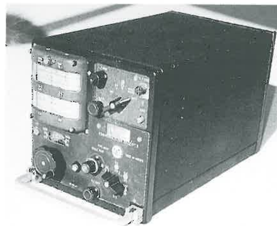
Marconi type AD94 Aircraft Receiver
