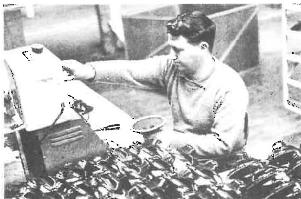
At left: AKRAD assembled and magnetised all its own loudspeaker (Barry Roycroft testing one).
