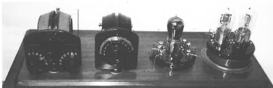
Early 1920s Atwater Kent Breadboard Radio. By selling the bakelite mounted pieces as a kitset to be assembled by the purchaser and not as a complete radio Atwater Kent avoided the high patent fees charged by RCA.
