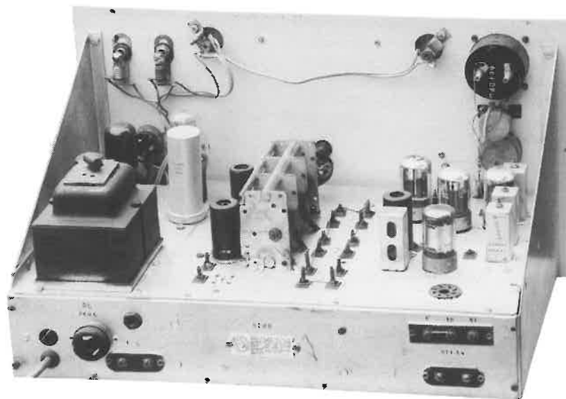
Q-Max G5/10X rear view. Note bizarre array of different valve types
