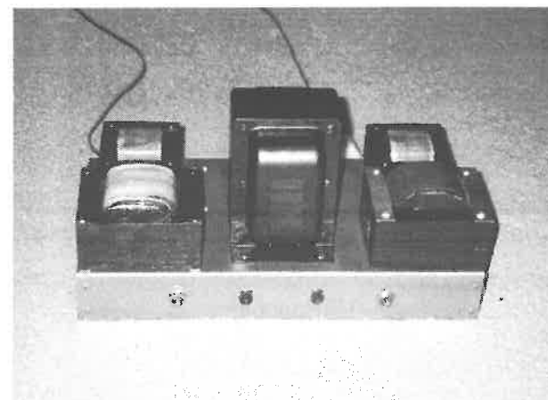
The largest item in the power supply is the very large HT filter choke.
