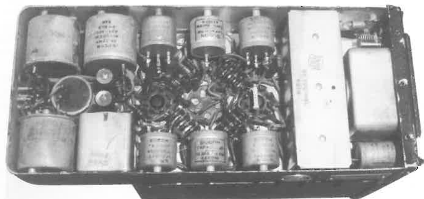
Under-chassis view of the 180 to 550 kc receiver which seems all totally original, apart from the replaced capacitors.
