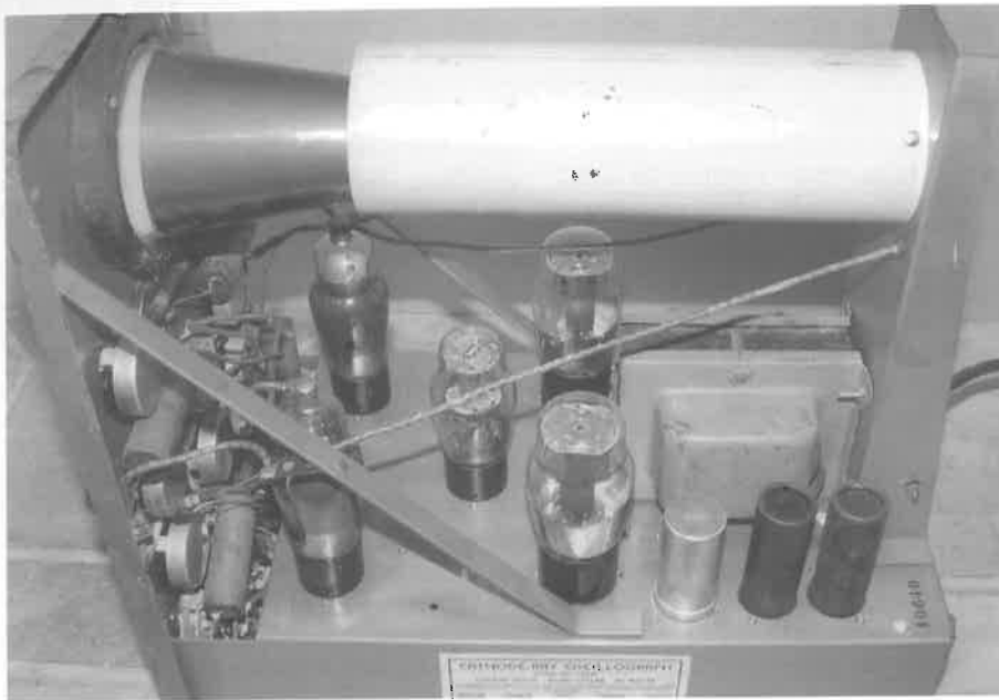
Above - Interior of RCA Oscillograph. Note the clean simple layout
