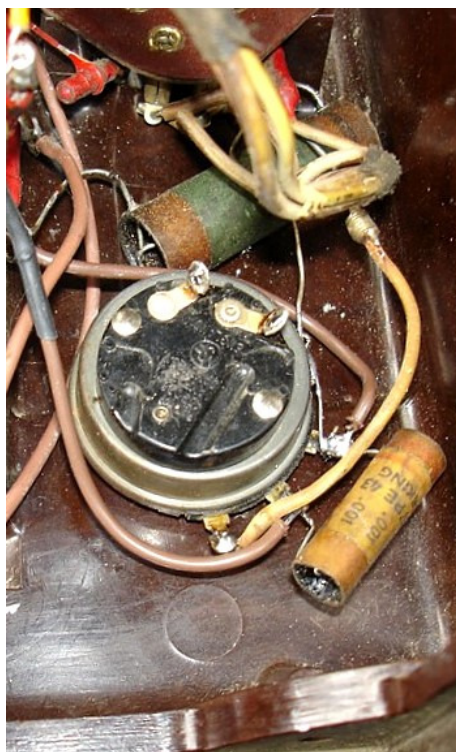
Left: Replacement volume control and restuffed capacitor shells.
