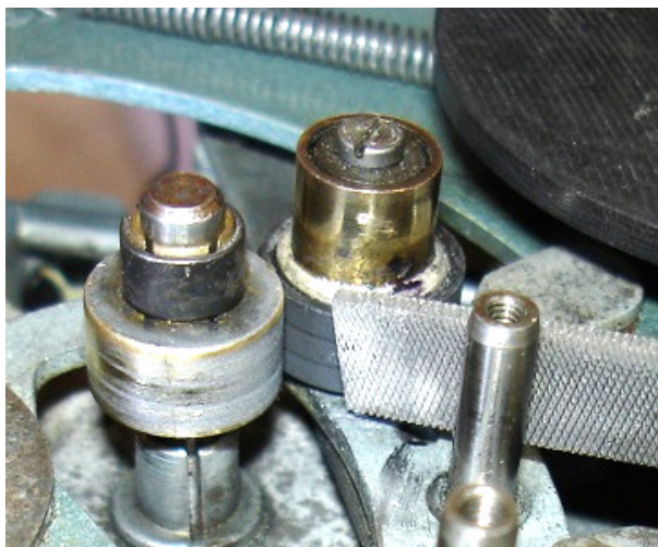
Left: Filing of the rubber O rings to adjust the turntable speed.
