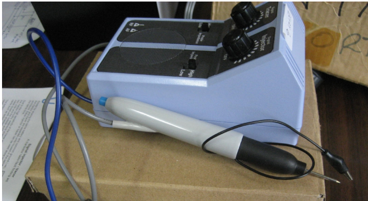
Left: The Signal Injector and Tracer from Colin Bowring even came complete with its own box.
