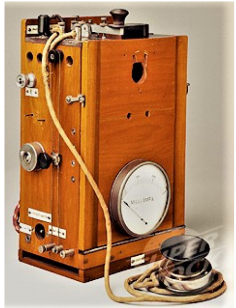
This combined radio telephony and telegraphy transmitter consists of microphone and key with internal Round valve.
