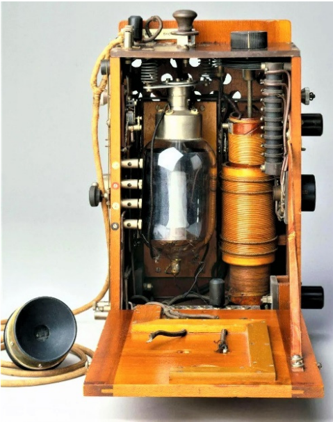
This combined radio telephony and telegraphy transmitter consists of microphone and key with internal Round valve.
