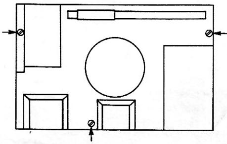
→ INDICATES CHASSIS SECURING SCREW
