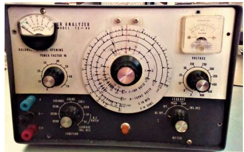
Normal TE-46 with magic eye at top, and modified with meter beneath.
