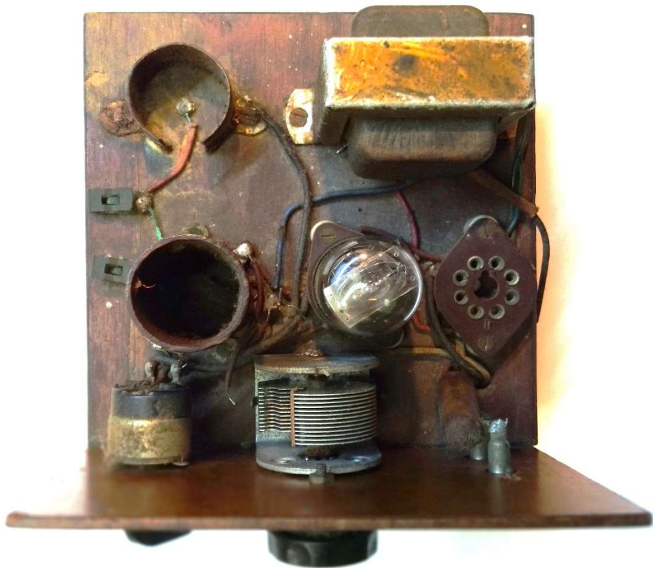
Editor's Two Valved layout with missing output tube.
